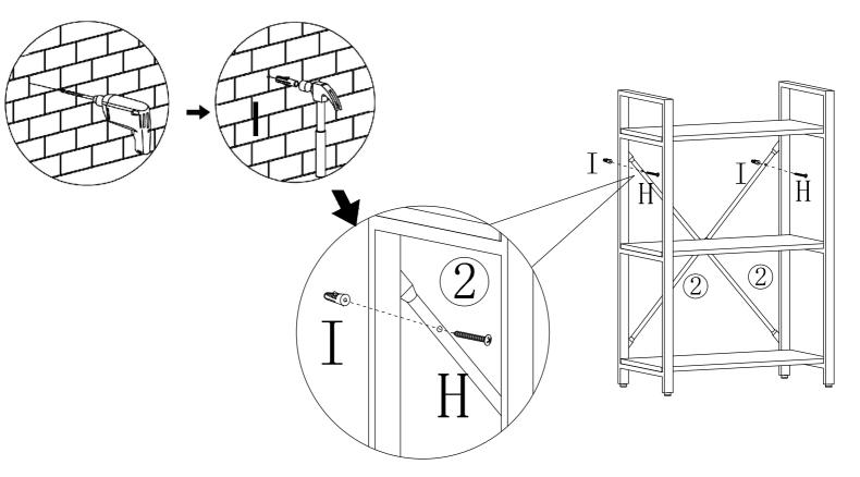
Important note: If you find the holes do not align together, you can loosen all the screws, and adjust the holes slightly. After all the holes were aligned together, you can fully tighten all the screws.
